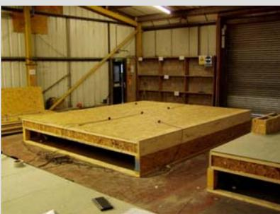
Fig 2: Floor systems supported on shallow wall panels
